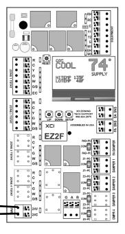
Connect the transformer to the 24V and 24C inputs on the zone control board.
