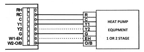
**BYPASS ELIMINATION ON SINGLE SPEED SYSTEMS:** When the board is set up for 1-speed outdoor unit, the board will energize **Y-2** to the equipment if more than one zone is calling. This allows the use of a 2-speed or multi-speed indoor unit with a **Y-1** and **Y-2** terminal. The indoor fan speeds can be set up to run on a lower speed on **Y-1**, and a higher speed on **Y-2**; eliminating the need for a bypass damper.
