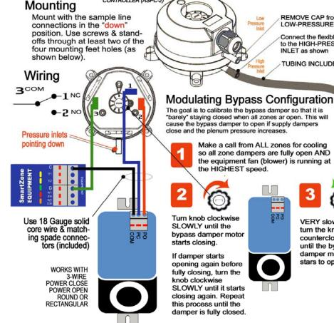
REMOVE CAP from LOW-PRESSURE INLET
